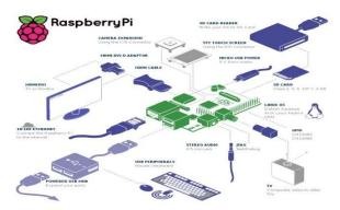
Figure 6.3:- Raspberry pi Architecture
