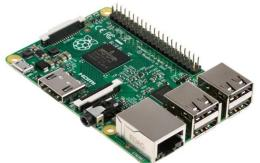
Figure 6.2:- Raspberry pi or ARM board
